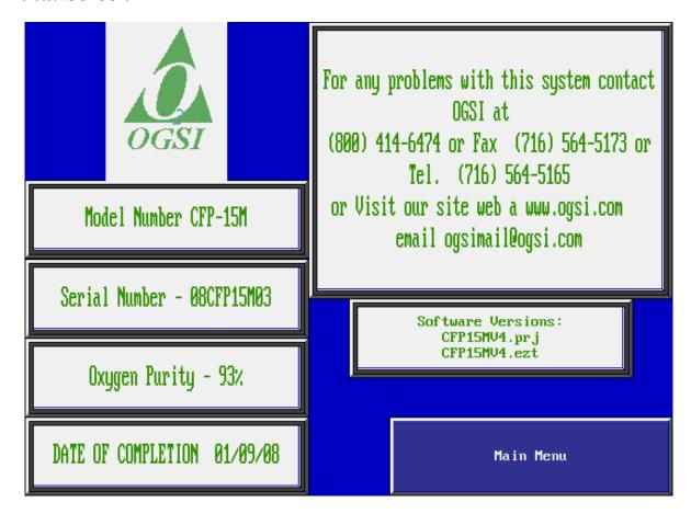
This screen displays information pertinent to the system, and manufacturer contact information. The Model Number of the Machine and its Serial Number are displayed along with the Date of Completion. The software versions for both the Programmable Controller and Touch Screen are also shown. During the course of normal maintenance, the company may offer to upgrade the software packages on the machine as improvements and modifications to it become available.
